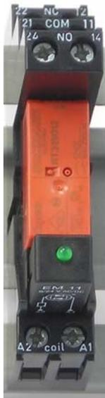
There are two screw terminals for each relay contact. Each can handle up to 8 amps. They are tied together internally.
