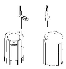
Fig. 4 Fixing the straining wire
