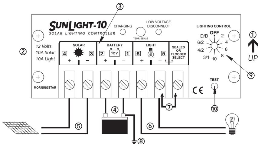
6. Connect the **LIGHT** last. If the red LED indicator lights, the battery capacity is low and should be charged before completing the system installation (Refer to Section 6.4).
