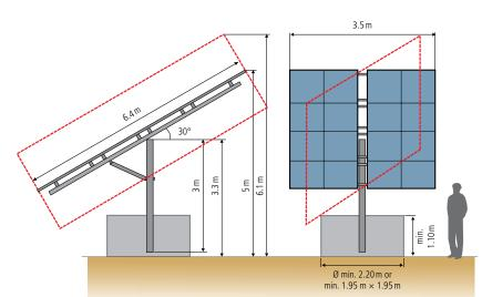
Example: system dimensions with 16 PV modules, c.  $1.6 \,\mathrm{m} \times 0.8 \,\mathrm{m}$
