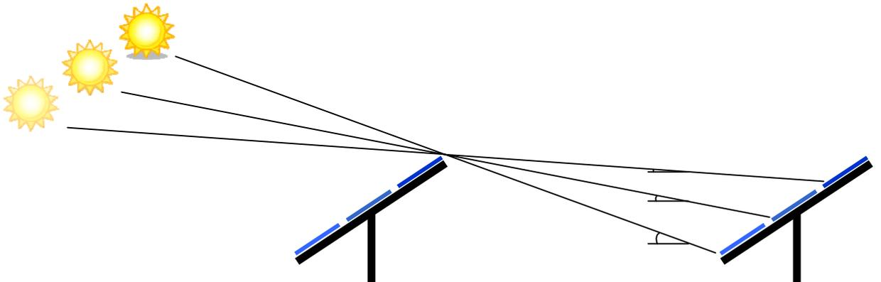
**Figure 6 Shading on modules**
