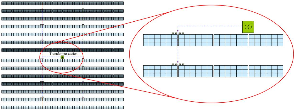
**Figure 4 PV field layout with inverters being distributed**
