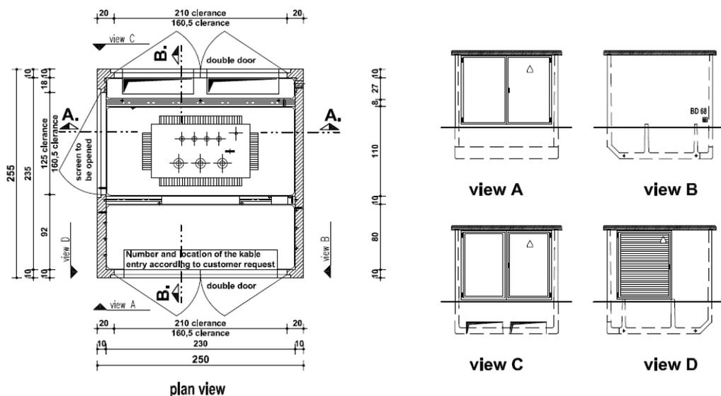
**Figure 5 Transformer station**
