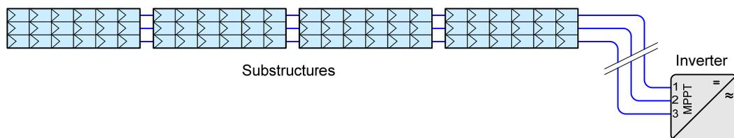
**Figure 2 Module wiring based on crystalline modules**
