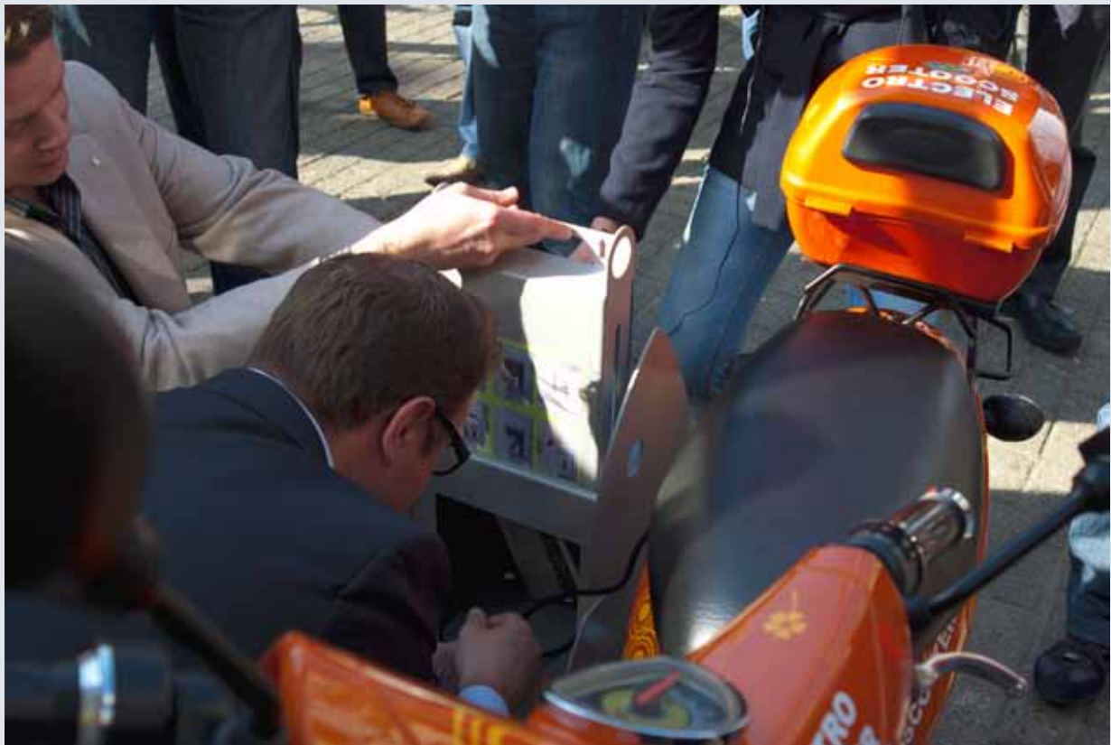
Photo 5: After the electrical scooter is connected, the battery can be charged.
