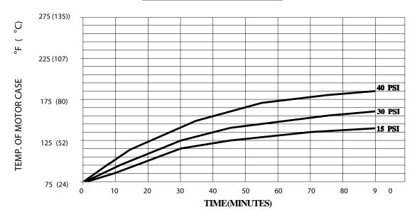
THIS GRAPH IS FOR USEAS A DESIGN GUIDE. IT IS BASED ON RUNNING CONTINUOUSLY WITH AN AMBIENT TEMPERATURE OF  $75^{\circ}$  F IN STILL AIR.
