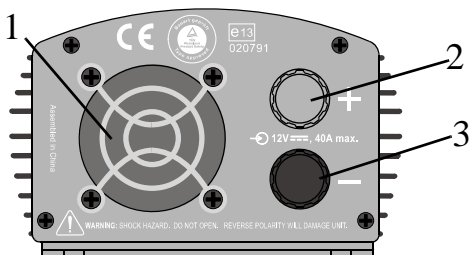
Figure 5 DC Panel on the XPower 300
