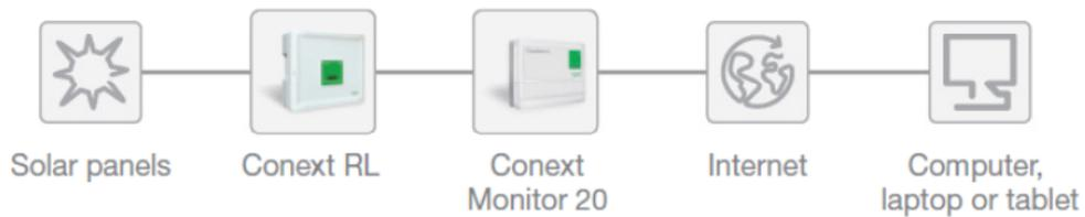
**Figure 7 – Remote monitoring option for Conext RL: Conext Monitor 20**
